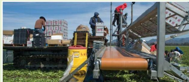
The boxes of celery move on conveyor belts just behind the washing and packing tables to the middle of the staging area, where they are stacked on the
